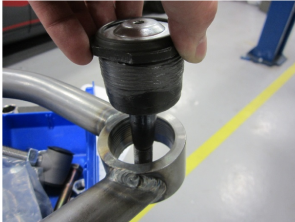
Installing Ball Joint
