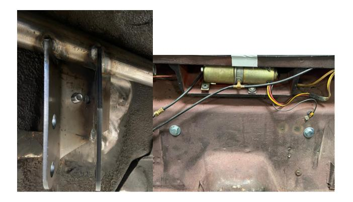
Next you will locate the rear shock mount saddles. Note there is a right and a left, make sure the shocks when installed angle inboard towards the center of the car. The saddles are located in between the stock shock mount crossmember. Some trimming may be required to the edge of the crossmember.
