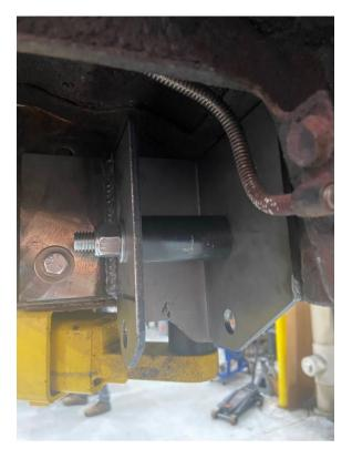
You can now install the lower and upper links. The lower links use the spacer at the outside of the link locating the front of the link inboard near the frame rail.
