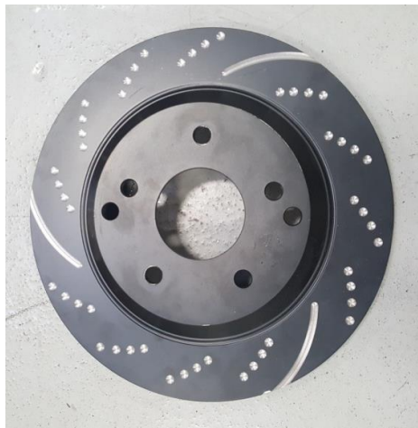
Dimple Drilled & Slotted Rotor, Fig. 76
