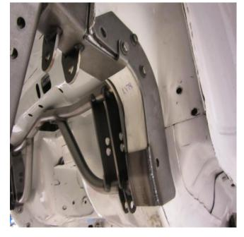
4) Drill the two 3/8" holes. Start with a 1/8" drill bit from the outside then with a 3/8" drill bit finish drilling the hole from the inside. Secure the bracket with  $(3/8-16 \times 1-1/4 \text{ bolts})$ , nuts and washer
