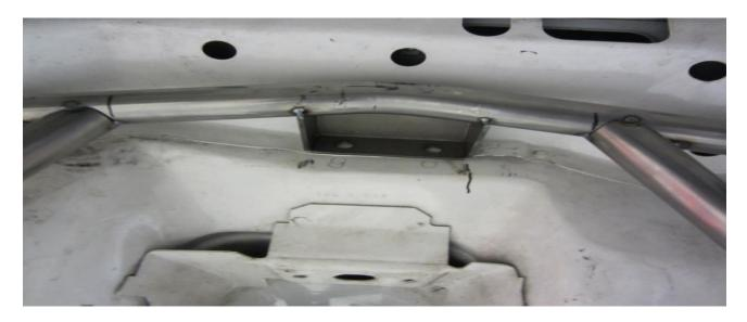
5) Install the left and right saddles. They locate off the factory bump stops but only the lower back 3/8 bolts will be used. Make sure the saddles are flat on the frame rail and hold the saddles in place with a vise clamp / c-clamp. Drill the six 1/2" holes though the frame.
