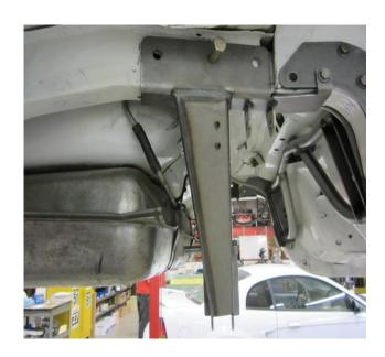
6) Install the six  $1/2-13 \times 4$ " bolts with washers, nylock nuts and leave them lose for now.
