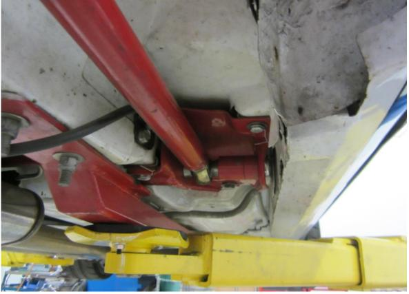
10) Once the links are installed install the panhard bar using the two lowest hoes as a starting point. See picture below.
