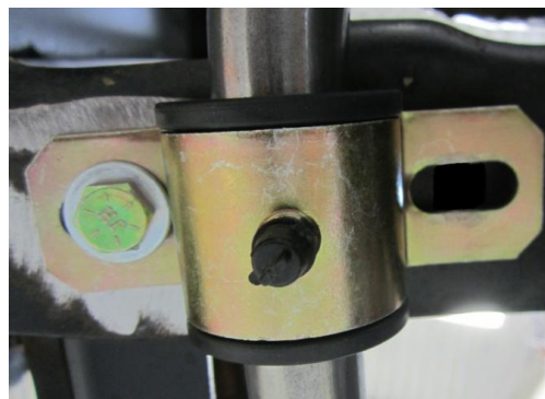
Bolt Installed, Centered On Bracket
