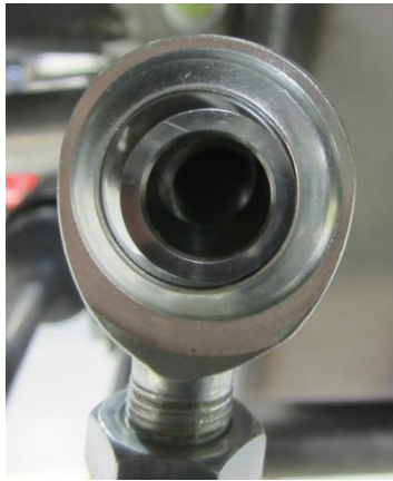
Rod End Not Fully Aligned
