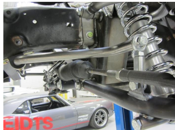
Rod Ends Installed, Drivers Side Wheel Well
