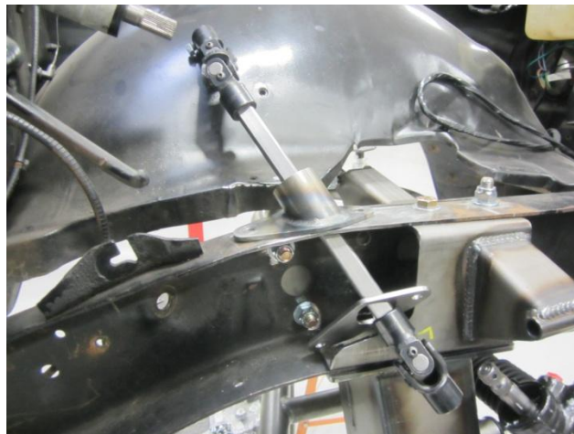
Bearing Mount, & Steering Shaft Plate Loose, Installing Linkage Figure 7
