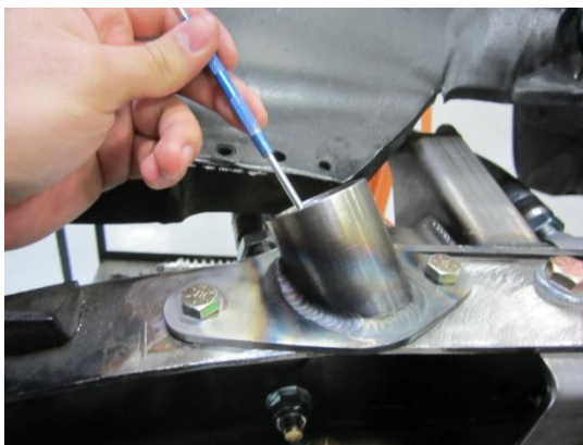
Scribing Hole Inside Bearing Mount
