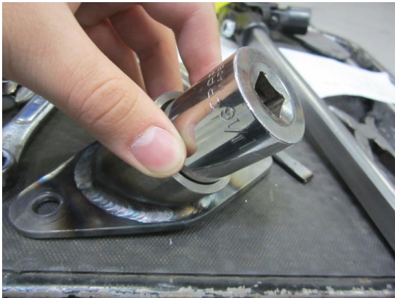
Driving In Spherical Bearing with 1 \frac{1}{16} " Socket
