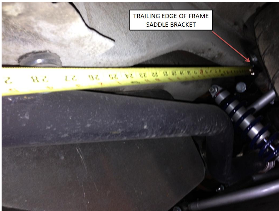
Figure 7. Passenger side Frame Saddle measurement
