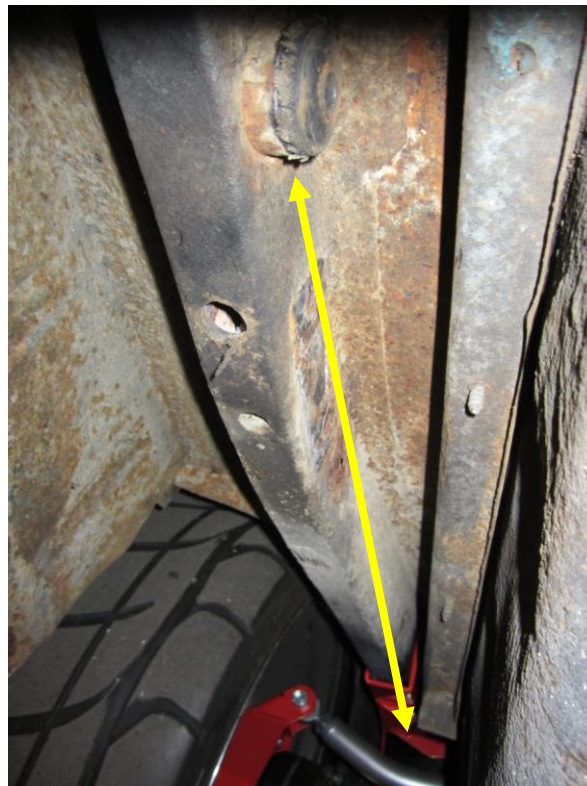
Figure 7. Measure between the edge of the rear leaf spring shackle mount and the rear edge of the frame rail saddle
