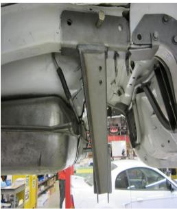
6) Install the six  $1/2-13 \times 3-1/2$  bolts with washers, nylock nuts and leave them lose for now.
