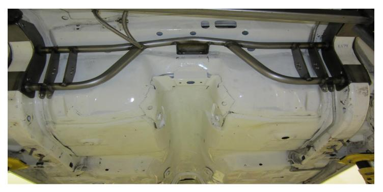
3) Locate the cross member using the factory bump stop nut plate with six  $(3/8-16 \times 1^{\circ})$  bolts and 3/8 washers) Drill the four  $1/2^{\circ}$  holes though the frame rail and use  $(1/2-13 \times 3-1/2)$  bolts, nuts and  $\frac{1}{2}$  washers) Making sure not to crush the frame rail when tightening the bolts.
