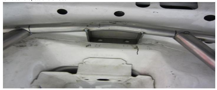
5) Install the left and right saddles. They locate off the factory bump stops but only the lower back 3/8 bolts will be used. Make sure the saddles are flat agented the frame rail and hold the saddles in place with a vise clamp / c-clamp. Drill the six 1/2" holes though the frame.
