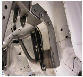
4) Drill the two 3/8" holes. Start with a 1/8" drill bit from the outside then with a 3/8" drill bit finish drilling the hole from the inside. Secure the bracket with  $(3/8-16 \times 1-1/4 \text{ bolts})$ , nuts and washer) Use the inner reinforcement plate on the inside.
