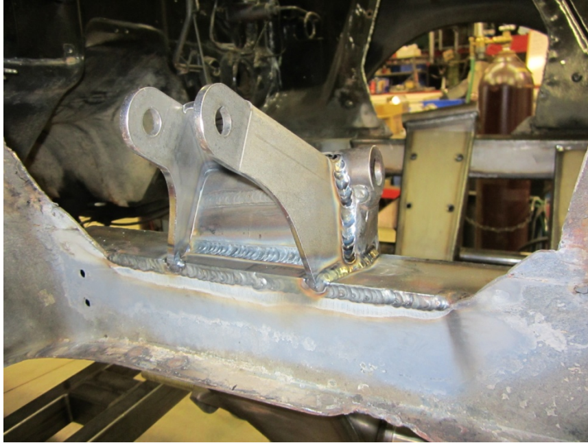
Figure 6. Fully welded Upper Shock Mount (Passenger Side)
