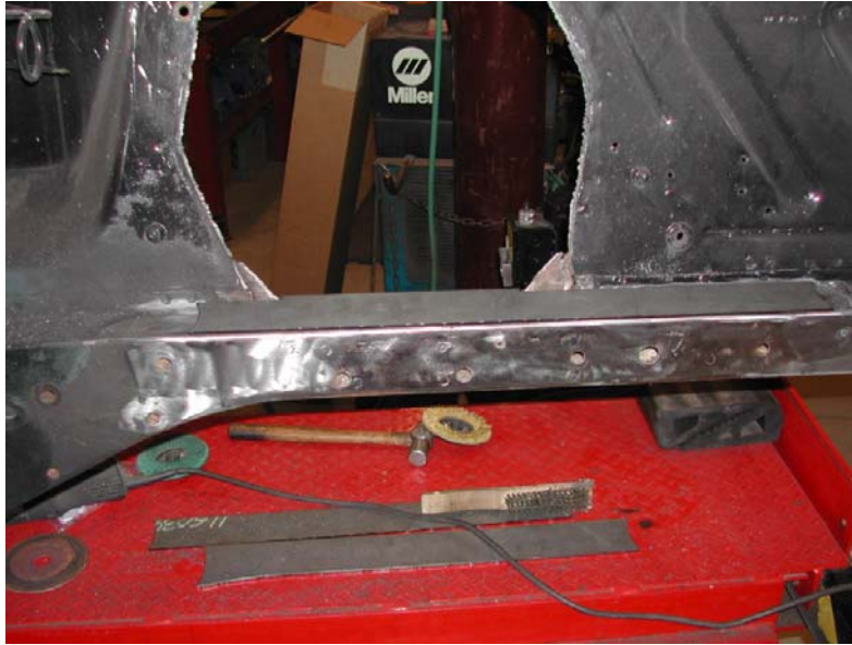
Figure 2. Driver Side Frame Rails ready for boxing plate installation
