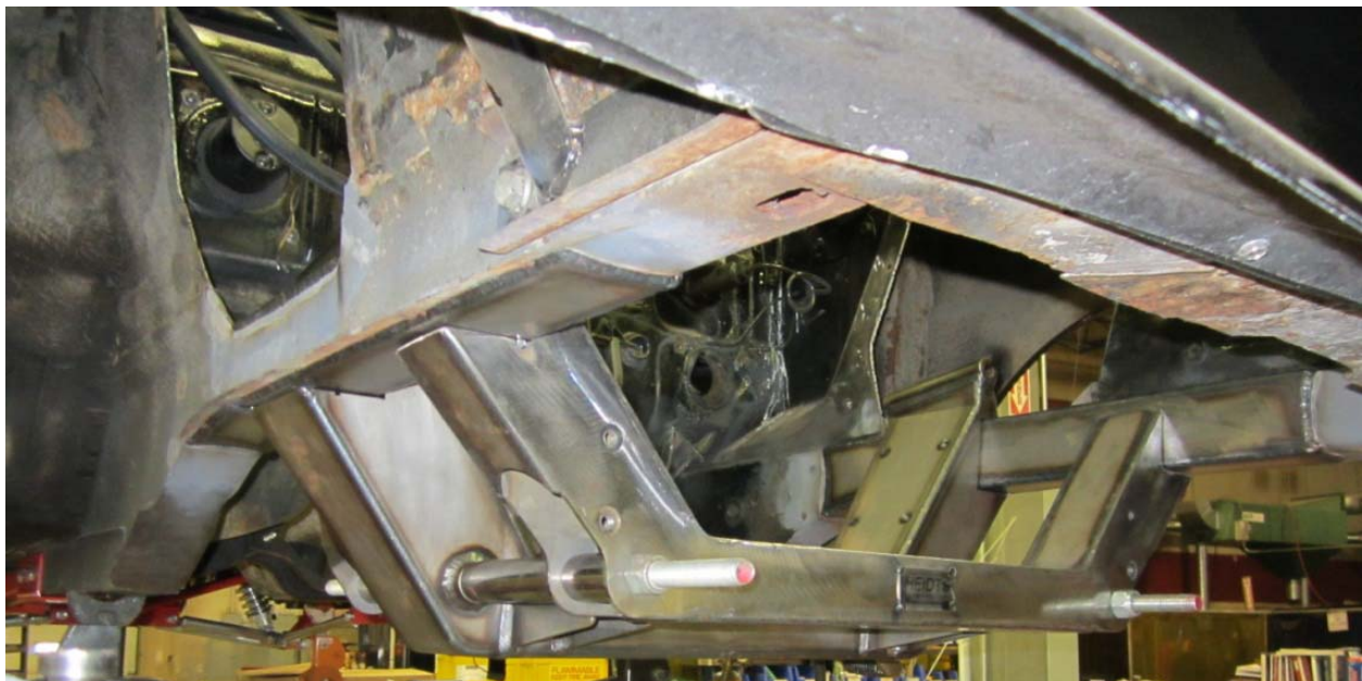
Figure 5. Front Crossmember installed using supplied spacer kit
